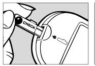
Insert the Check Strip fully into the Meter. Wait 10 seconds for the memory sequence to begin. NOTE: You may also use a Test Strip to delete all test results from memory. However, you must wait 3 minutes for the memory sequence to begin. When you see the memory sequence begin, proceed to Steps 2 and 3.
